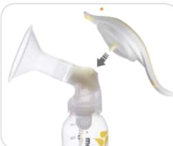
Insert base of handle assembly into opening on connector until it locks into place.
